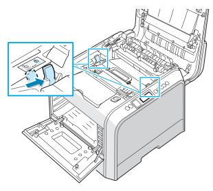
**CAUTION**: If you open the left cover for a few minutes, the imaging unit can be exposed to light. This causes damage to the imaging unit.
